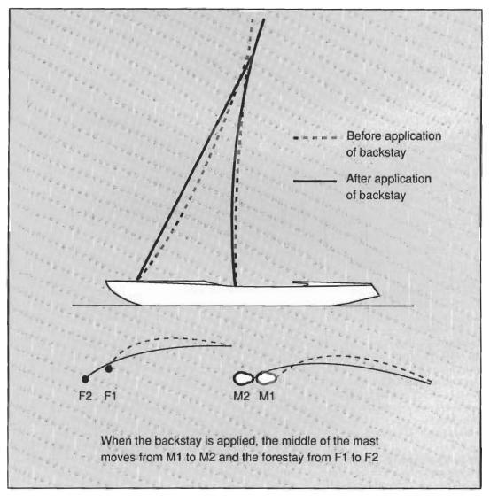
moves aft causing a board to head up and a keelboat to develop weather helm.
